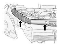
Detach fasteners and lift off the panel that covers the radiator cap. Remove the radiator pressure cap when the cooling system, including the upper radiator hose, is no longer hot.
